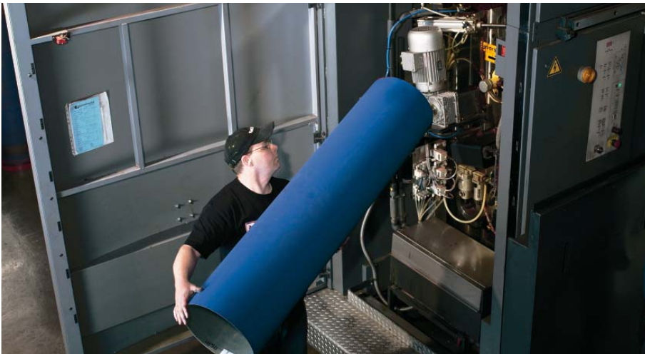
Gapless blankets slide in through the side frame and can be changed in less than two minutes.
